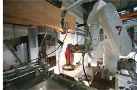
Fig. 5. Clean-up of the interbucket spaces.
