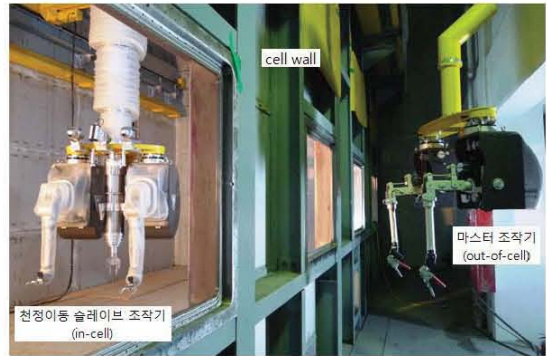
Fig. 3. Servo-manipulator installed at the transporter
