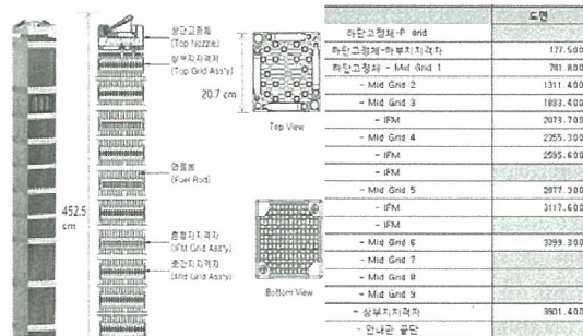
Fig. 2. 16 x 16 PWR SF assembly dimension.
