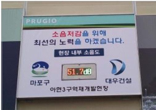
Figure 1. Construction Noise Board
