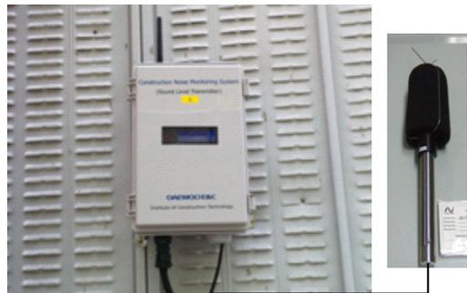
Figure 2. Sound Level Meter with wireless data transmitter
