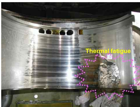
Fig 1. Thermal fatigue damage of bearing
