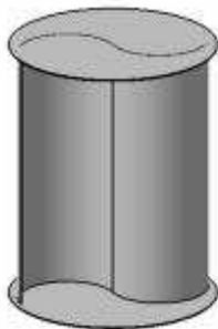
Fig. 1 Configuration of a Savonius wind turbine
