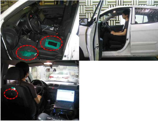
Fig. 4 Photo illustration for the sensor location and driver position for the vibration measurement
