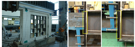
Figure 1 Specimen setting and damping rubber
