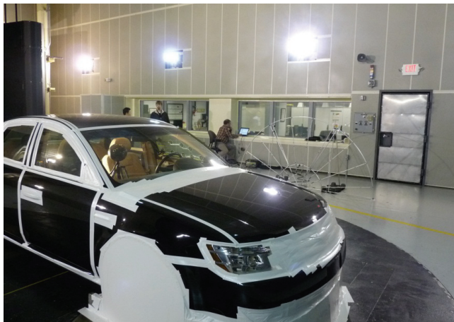
Fig. 5 – Wind tunnel with taped vehicle on rotating plate used to adjust yaw angle. Spherical Beamformer in the cabin, and Half Wheel Beamforming array at 3.8 m distance (0 degree yaw)
