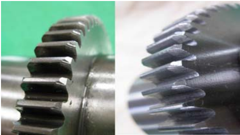
Fig. 2 Gear tooth weaned by misalignment
