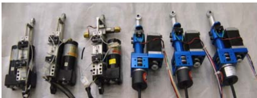
Figure 4 Pitch Actuator(Left:Old, Right:New)
