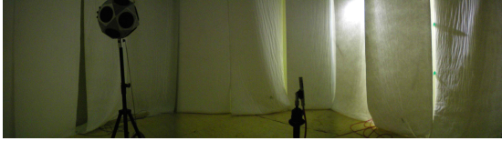
(a) Sound absorber installed on 6 faces of room
