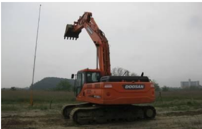
Fig 1. Radiated Noise Measurement According to 2000/14/EC
