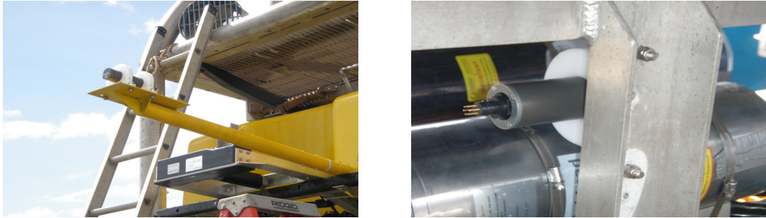
Fig. 2. (a) Magnetometer Sensor on ROV (b) Data Logger on ROV
