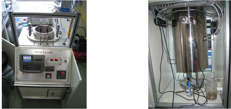
Fig. 1. Engineered PCC mixing batch.
