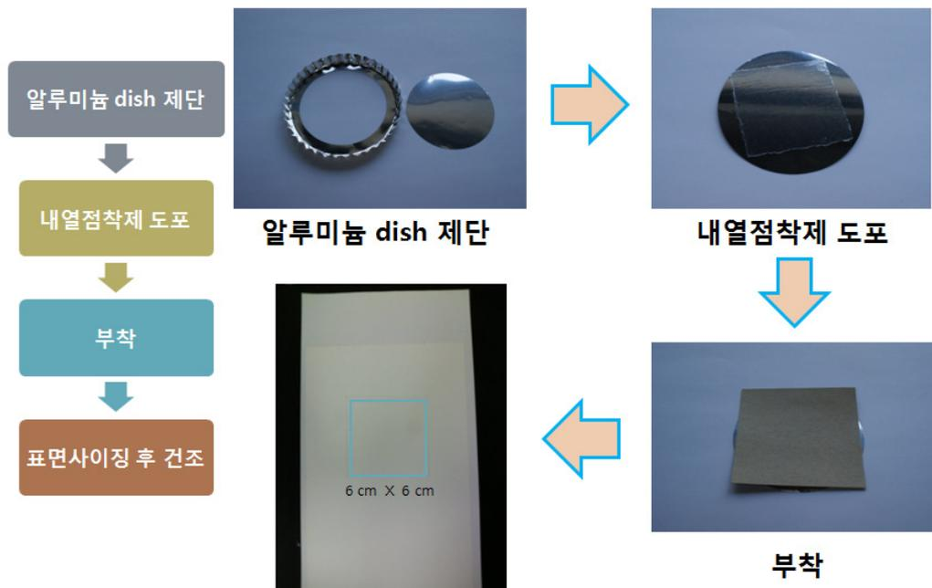
Fig. 1. Flow chart of the measurement on dryness of surfaced sized paper.
