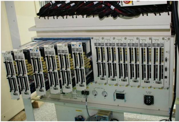
Fig. 3 Modules of Bidirectional DC/DC Converters.
