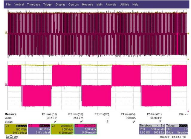
Fig. 5 Experimental waveforms of DC-link voltage(C1) and junction voltage(C2)
