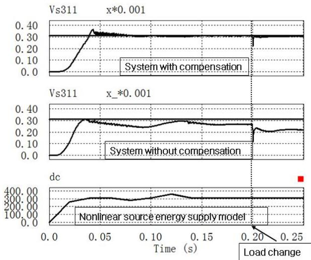
Fig. 3 system comparing under DQ coordinate
