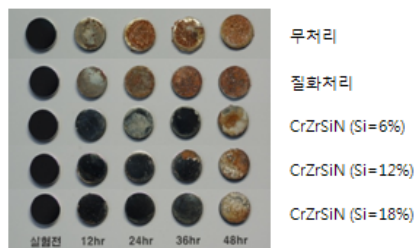
Fig. 1. Salt spray test of CrZrSiN thin films
