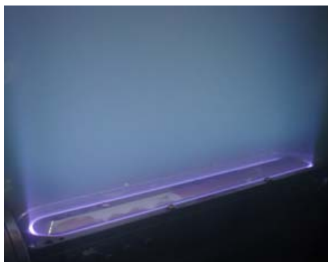
Fig. 1. Closed drift linear Ion source (Anode layer type)
