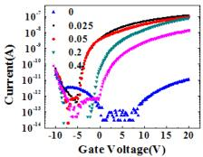
Moon et al..[4] These decreases shift the  $V_{th}$  toward a positive direction, which is controlled by carrier concentration in the channel.<sup>19,20</sup> Also, these systematic variations in the transfer curve including the  $V_{th}$  shift and the off-current reduction are possibly caused by the addition of Si. As Si content increasing, it is expected to suppress carrier generation through reducing oxygen vacancy formation and hence help to achieve lower on-current.
