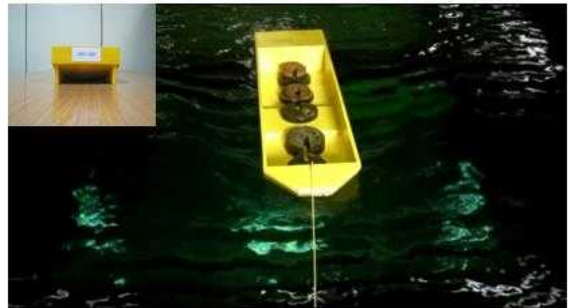
Slewing motion of KNU-002( l = 1L , No bridle, V_s = 7.0 kts, Side skeg)
