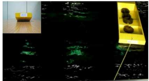
Slewing motion of KNU-001 ( l = 1L , No bridle, V_s = 7.0 kts, No skeg)
