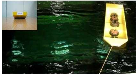
Slewing motion of KNU-002( l = 1L , No bridle, V_s = 7.0 kts, No skeg)
