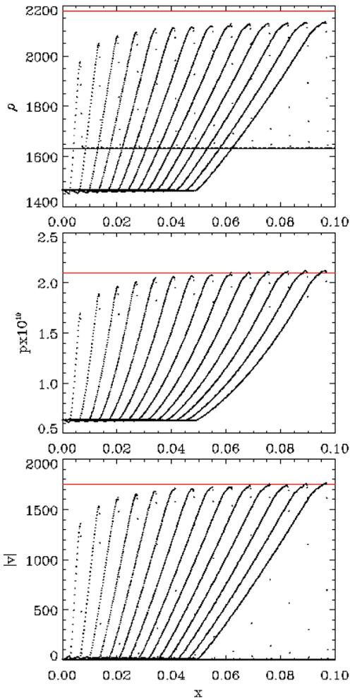
Fig. 2 Density, pressure and velocity profiles along the one dimensional TNT slab. The red lines indicate the experimental values for the peak values of the density, pressure and velocity at the trailing edge of the thin reaction zone
