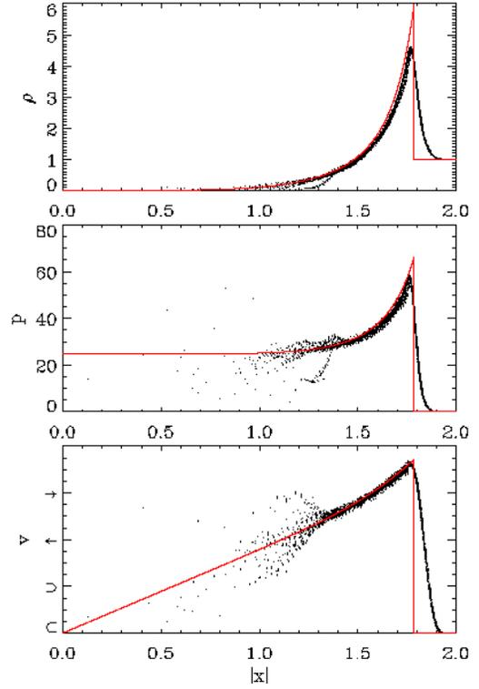
Fig.1 Results of the Sedov blast wave test at a time  $t = 0.1$ . The black dots represent the SPH result and the red lines show the semi-analytic solution provided by Sedov
