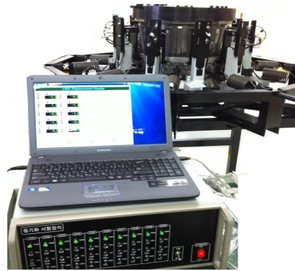
Fig. 1 Synchronization test system of variable nozzle
