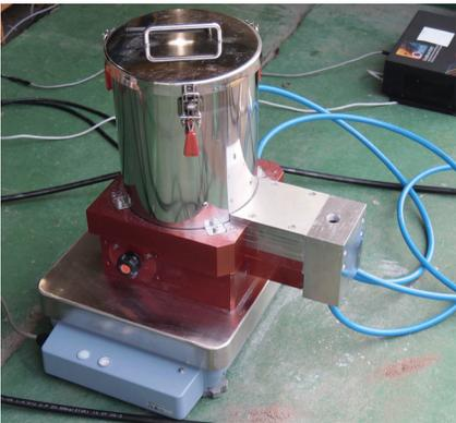
Fig. 5 Photograph of aluminum feeder
