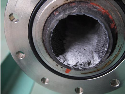
Fig. 8 Accumulated slag of alumina
