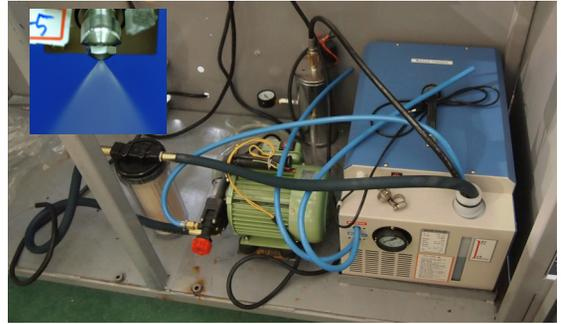
Fig. 6 Water supply device and pressure swirl type water injector
