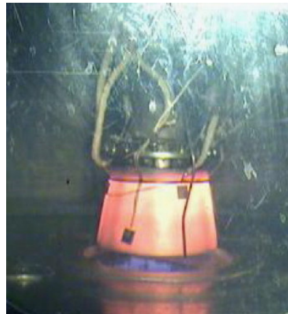
Fig. 6 Firing Test of 11D58M Engine [14]
