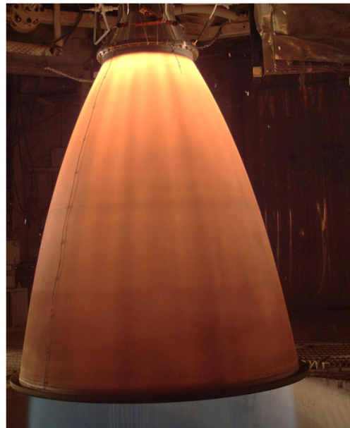
Fig. 3 Altitude Testing of Methane Engine of Aerojet and GenCorp. [8]
