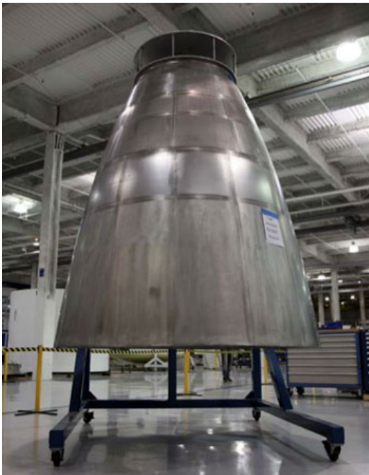
Fig. 2 Nozzle Extension of Merlin Engine [6]
