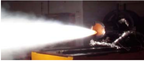
Fig. 2 Flame shape at the exit of control valve
