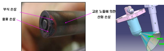
Fig. 10 Damaged igniter tip and relative igniter position for fuel spray
