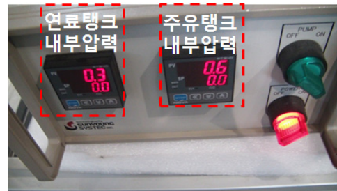
Fig. 8 Tank Pressure after Refueling
