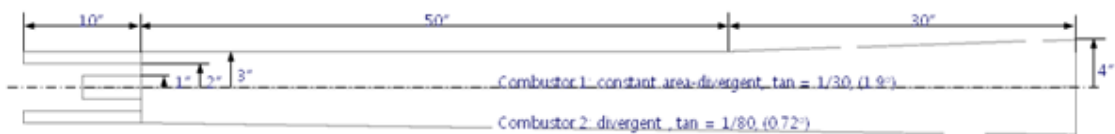
Fig. 2 Computational domain of the supersonic combustion flow field in DCR: (upper) model combustor 1 with constant area duct followed by a diverging duct, (lower) model combustor 2 with divergent duct.
