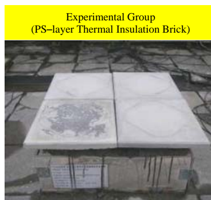
Fig. 9 The experimental group in the experiment of insulation performance
