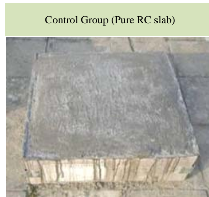
Fig. 8 The control group in the experiment of insulation performance
