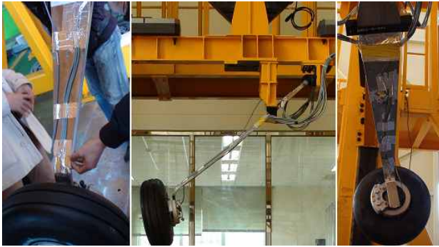
Fig. 2 Test Specimen of the Drop Test
