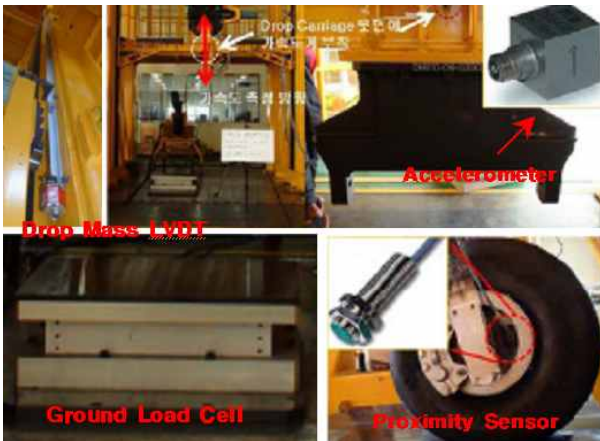
Fig. 6 Sensors for Drop Test
