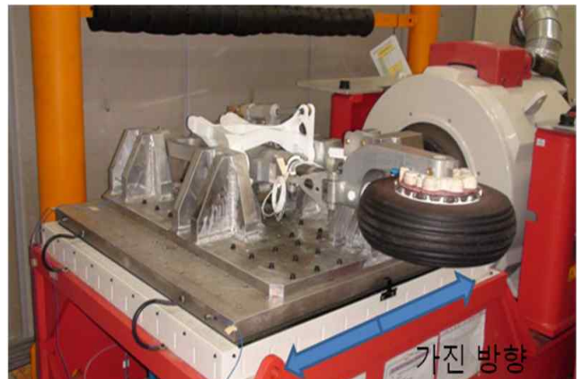
Figure 4 Test set-up for the MLG, X-axis vibration
