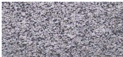
(b) Stir zone of FSW, (200x)
