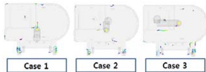
Fig. 5 Analysis result for weld lines
