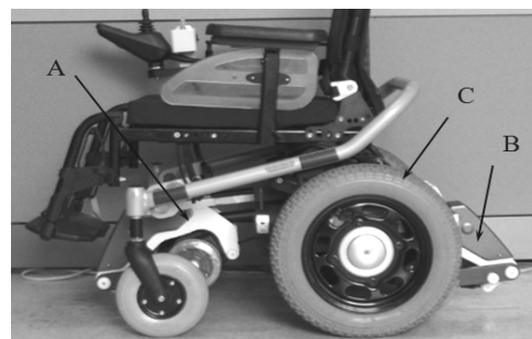
Fig. 2 Photographs of the curb-climbing wheelchair : A, B Curb-climbing aid; C, Driving wheel.
