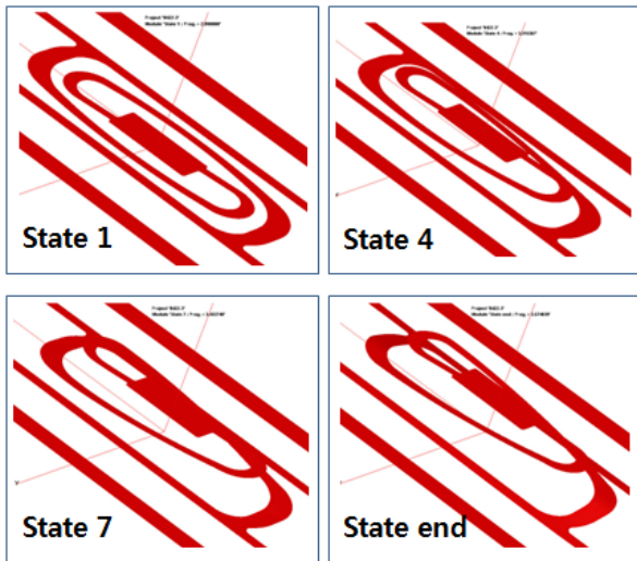
Fig. 3 Process procedure of bending
