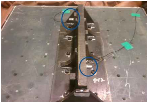
Fig. 2 Installation of accelerometer
