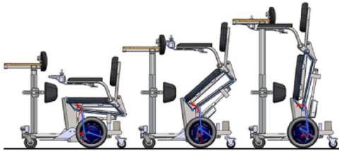
Fig. 2 Moving process from seating to standing of in-wheel motor axle by links connected 4-bar link mechanism
