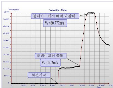
Fig. 3 Averaged velocity variation of shot ball during simulation
