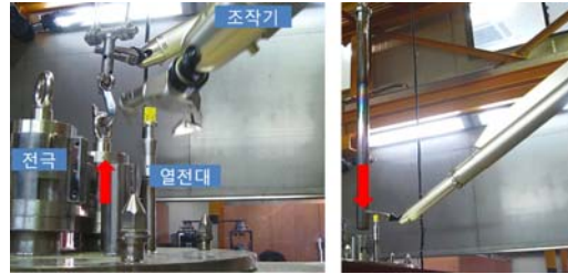
Fig. 4 Example of tele-operation task in the 1/8 scale Mock-up Facility (Cathode electrode handling)
