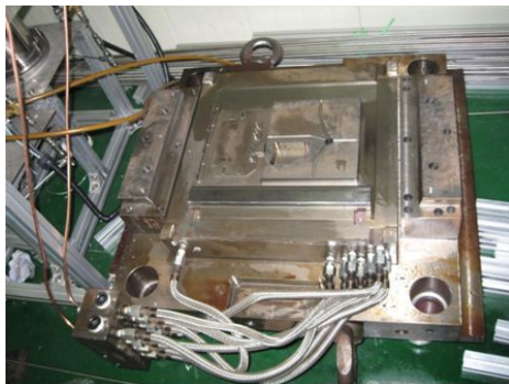
Fig. 4 Efficiency test mold for injection mold temperature control system
