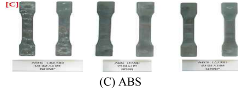
Fig. 2 Appearance of the injection molded specimen using PET and PC/ABS and ABS
