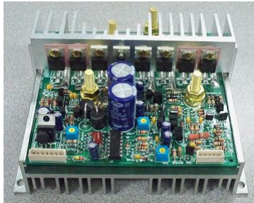
Fig 3. Main DC Motor Controller
