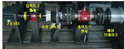
Fig. 5 Transmission efficiency measurement equipment
