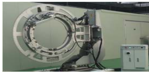
Fig. 1 Developed Hardware Platform and its Controller of Medical Robot for Diagnostic Imaging Purpose
