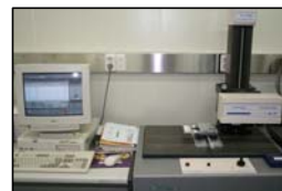
Fig. 2 Photograph of measuring instrument (Form Talysurf Series2)
