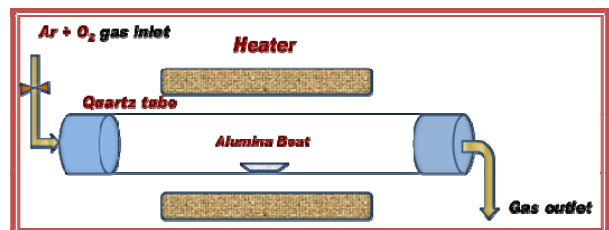
Fig. 1 Experimental setup for growth of Cu doped ZnO nanorods.
