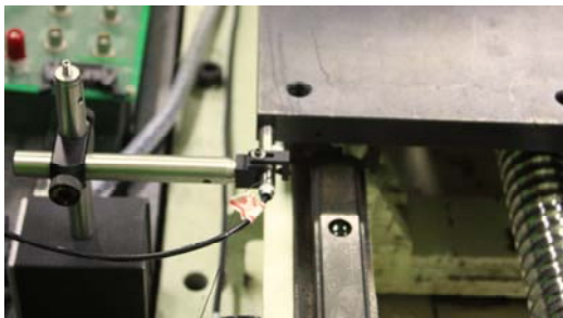
(b) Attachment of a capacitive displacement sensor
